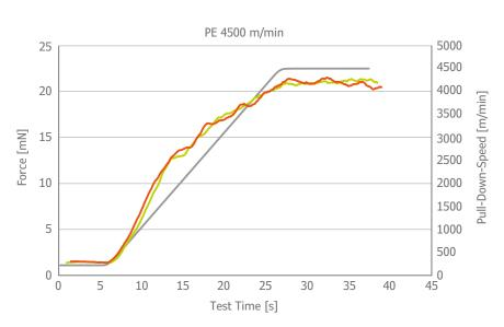
A typical test method is the ramp test up to the desired pull-off speed with a short speed holding phase. In the case of a mono filament, the material can also be wound up at the pull-off wheel without any appreciable increase in speed.
