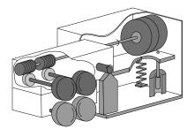
The functional diagram shows the RHEOTENS 71.97 with tandem pull-off wheels, which can also be retrofitted to older devices.
