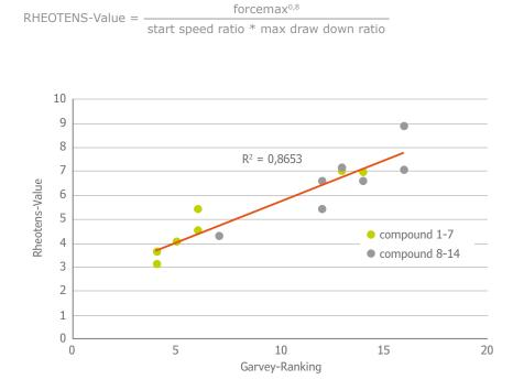
For elastomers, this results in a good correlation to the extrudate quality manually evaluated using the complex extrusion test with the Gravey die, which is also more prone to errors due to this manual evaluation.
