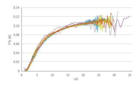
A further normalization determines the influence of the die geometry and the length of the spinning line. Finally, all 16 RHEOTENS curves are reduced to a single elongation curve, the RHEOTENS Grand Master Curve, by scaling the pull-off force F and elongation; now based on:
