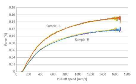
According to the manufacturer, sample B indicates a somewhat broader molecular mass distribution (Mw/Mn=11.1) than sample E (Mw/Mn=10). The RHEOTENS curves, each reproduced three times, indicate a clear increase in the melt strength of sample B compared to sample E.
