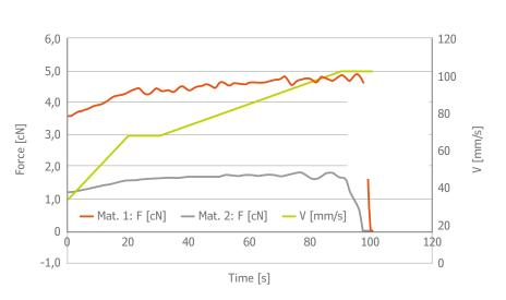
The following comparison shows the considerably higher selectivity of the test method compared to the pure melt index measurement. The simple operation, short measuring time and low speeds make this method particularly suitable for quality assurance during compound release or in incoming goods inspections.
