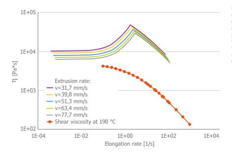
Using a simple analytical model, the effective elongational viscosity function can now be determined. As a function of the elongational rate, it is composed, depending on the extrusion history, of the "visco-elastic start-up" with increasing elongational viscosity and the purely viscous elongation with decreasing viscosity.
