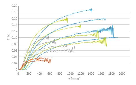
In the technical elongation diagram, the speed or velocity v is a relative measure of the "elongation" of the melt. The maximum force F delivers a relative value for the tensile strength. The simple RHEOTENS experiment is first of all a complex function of the polymer property, the die geometry, the length of the spinning line and the extrusion history.
